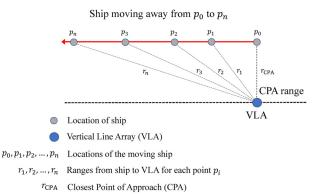
FIG. 2. (Color online) A schematic showing an acoustic source moving from right to left ( $p_0$  to  $p_n$ ) relative to a vertical line array (VLA) depicting the CPA range. The points  $p_1, p_2, ..., p_n$  show the different positions relative to a VLA when the ship is moving along the red track.
