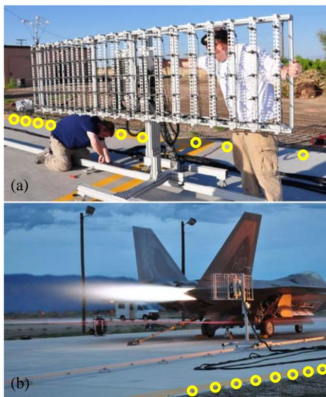
Fig. 2—Two views of the 90-channel field array rig mounted to a guide rail. Reference microphone locations on the ground are marked with yellow circles.
