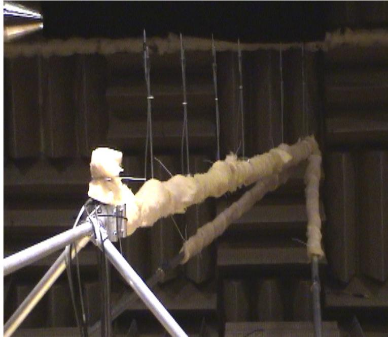
Figure 1. Photograph showing nozzle and microphone boom in the NCPA anechoic jet noise facility.
