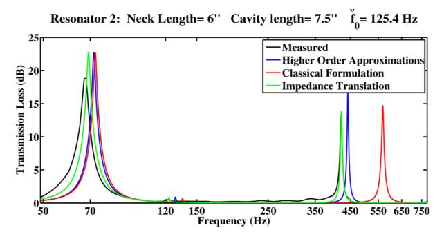
Fig. 6 - Comparison of transmission loss for measured and modeled data.
