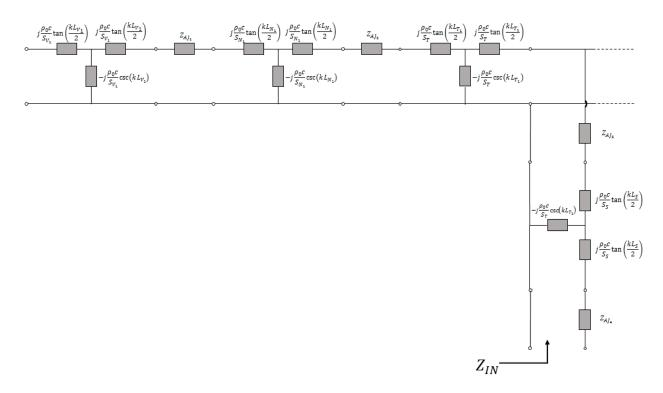
*Fig. 5 - Equivalent circuit of the resonator array. The dots to the right of the circuit represent the branch leading to the second resonator. The branch that is not pictured is a mirror image of the first resonator branch.*
