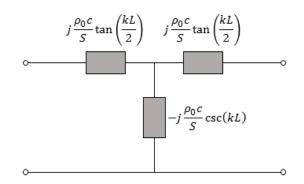
*Fig. 2 - T-network representing the impedance translation theorem over a distance L with cross-sectional area S.*
