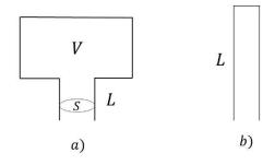
Fig. 1 - A simple representation of a) a Helmholtz resonator and b) a quarter-wave tube.
