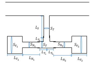
Fig. 3 - Schematic of the resonator array under test.
