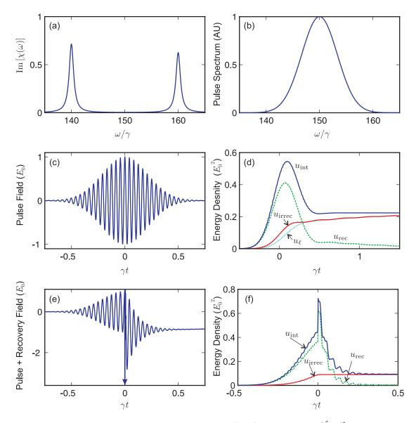
FIG. 1. (Color online) Quantities related to the parameters in (55). (a)  $\text{Im}[\chi(\omega)]$ . (b) The spectrum  $|\hat{E}(\omega)|^2$  of pulse field (arbitrary units). (c) Time evolution of electric field. (d) Energy densities associated with the pulse-medium interaction for the field in (c). (e) The field with a recovery field appended after t=0. (f) Energy densities associated with the field in (e).
