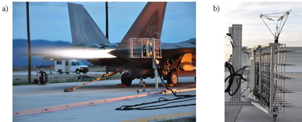
**Figure A-1. (a) F-22 engine firing with rig and probe in place, and (b) close-up of the intensity probe positioned on top of the microphone array. The array and probe took measurements at several locations along guide rails while the engine was cycled through four power conditions.**
