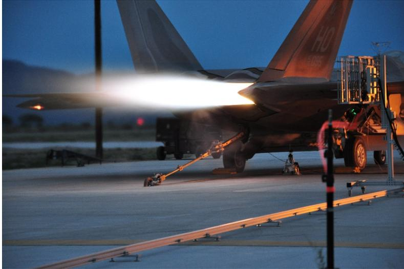
Figure 1-1. Measurement setup, with F-22 tethered to concrete run-up pad. The rectangular microphone rig is visible on the right, atop an aluminum guide rail.
