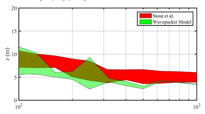
Figure 5.10. Comparison of the estimated maximum equivalent source region from the ray-tracing method employed by Stout et al. and the optimized wavepacket ESM for the F-22 when a single engine was operated at afterburner power.
