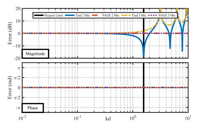
Figure 3.7. The relative error in the specific acoustic impedance for a plane wave using the different probes and processing methods. The top plot shows the magnitude error, and the bottom plot shows the discrepancy in phase.
