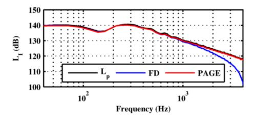
Figure 1.1. The sound intensity level  $(L_I)$  in a GEM-60 rocket noise field computed using the traditional or finite-difference method (FD) and the PAGE method. Both are compared to the sound pressure level  $(L_p)$ .
