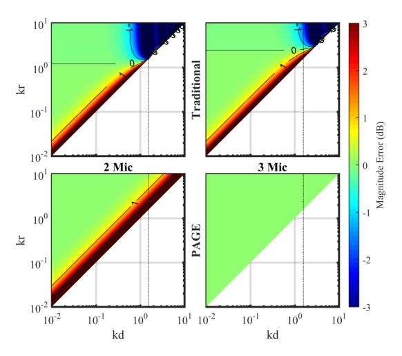
Figure 3.13. Active intensity relative error for the traditional and PAGE methods applied to two and three-microphone probes. The black line is the spatial Nyquist limit. The three-microphone PAGE case has no error in estimating active intensity for all values of kd and kr. The two-microphone probe is susceptible to bias error when the probe is only a few d from the source. The traditional method also breaks down for large values of kd.
