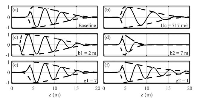
Figure 5.2. Various normalized wavepacket shapes. The baseline parameters are  $U_c = 478 \text{ m/s}$ ,  $b_1 = 4 \text{ m}$ ,  $b_2 = 14 \text{ m}$ ,  $g_1 = 14 \text{ m}$ , and  $g_2 = 2 \text{ m}$ . For the various plots (b)-(f), one parameter is changed from the baseline as indicated in the plot.
