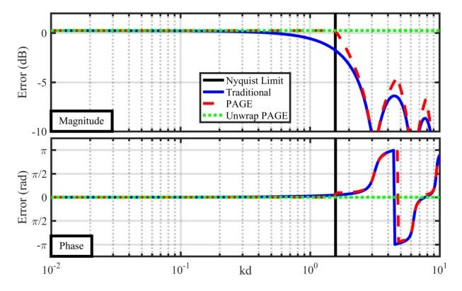
Figure 3.11. The computed magnitude and phase error of particle velocity for a monopole at a distance of r=4.3d. d=2 cm and is the spacing from one microphone to the center. The error for both the traditional method and PAGE methods for calculating particle velocity at the center of a two-microphone intensity probe are shown. The SNF indicates where the microphones are half a wavelength apart, making the phase between their measurements  $\pi$  radians different. All
