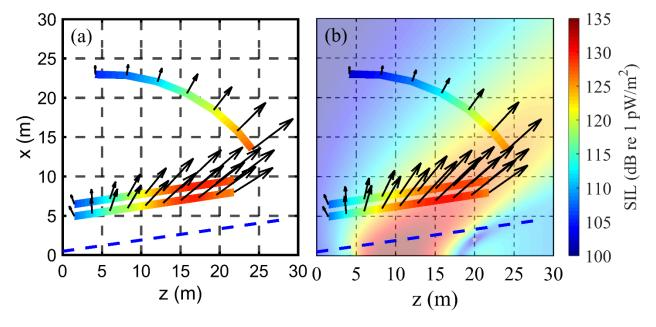
Figure 5.5. For 125 Hz and military engine condition, subplot (a) shows the measured afterburner acoustic intensity vectors, and subplot (b) shows the wavepacket-predicted intensity vectors. Subplot (b) has the wavepacket-predicted intensity level throughout the region. The dashed line indicates the approximate jet shear layer. The predicted levels inside the shear layer are not related to the turbulent flow and have no meaning.
