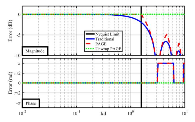
Figure 3.3. The computed magnitude and phase relative error  $(e_u + 1)$  of the complex particle velocity at the center of a two-microphone intensity probe from different methods. The SNF indicates where the complex particle velocity estimated from the microphones is  $\pi$  radians out of phase. Both the unwrapped and wrapped PAGE methods have the correct magnitude, but only the unwrapped PAGE method has the correct phase above the SNF.
