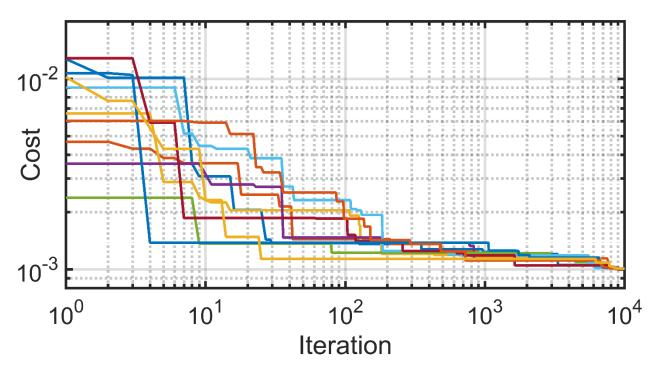
Figure 5.3. The various cost functions for military engine condition at 125 Hz for 10 different optimization runs.
