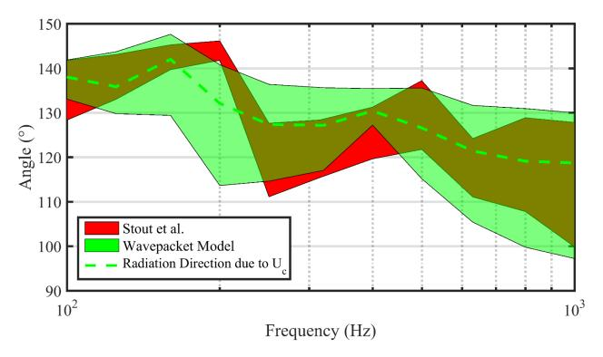
Figure 5.9. Comparison of the direction of the largest measured and wavepacket-predicted intensity vectors on plane 2 at military engine conditions. The dotted green line represents the peak radiation direction computed from the optimized convective velocity using Eq. 5.2.
