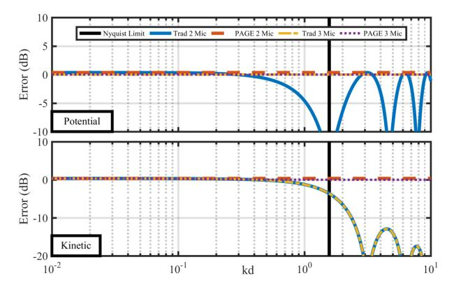
Figure 3.16. The energy density relative error when r = 4.3d. The top plot is the potential energy, and the bottom plot is the kinetic energy. The traditional method has error that oscillates above the Nyquist limit. The PAGE method shows constant bias errors. The bias error goes to 0 dB above the Nyquist limit for the three-microphone case.
