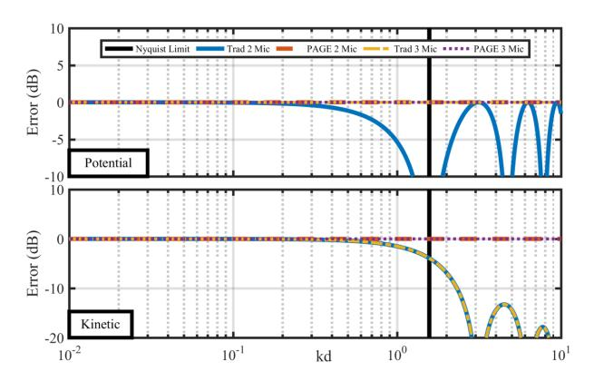
Figure 3.5. The relative error for estimates of the potential (top) and kinetic energy density (bottom) for a plane wave.
