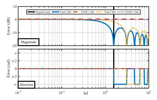
Figure 3.12. Active intensity relative error for different methods and probes for a monopole at a distance of r = 4.3d. d = 2 cm and is the spacing between the microphone and the center. The top plot shows the magnitude error and the bottom plot shows direction errors.
