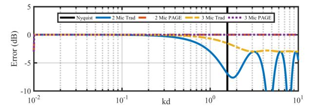
Figure 3.6. The relative error in the total energy density for a plane wave using the different probes and processing methods.
