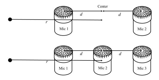
Figure 3.1. Schematic of the two-microphone one-dimensional probe (top) and the three-microphone probe (bottom) one-dimensional probe. r is the distance from the origin to the center of the probe, and d is the distance from the center of the probe to the outside microphones.
