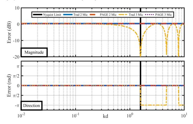
Figure 3.14. The reactive intensity relative error for r = 2d, d = 2 cm, and d is the distance between the center and an outer microphone. Bias error is present in all of the processing and probes depicted. The traditional method applied to three-microphone probe is frequency dependent in its error, as are both of the PAGE method estimates.
