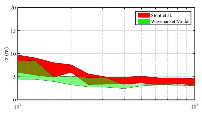
Figure 5.8. Comparison of the estimated maximum equivalent source regions from the ray-tracing method employed by Stout et al. and the optimized wavepacket ESM for the F-22 when a single engine was operated at military engine conditions
