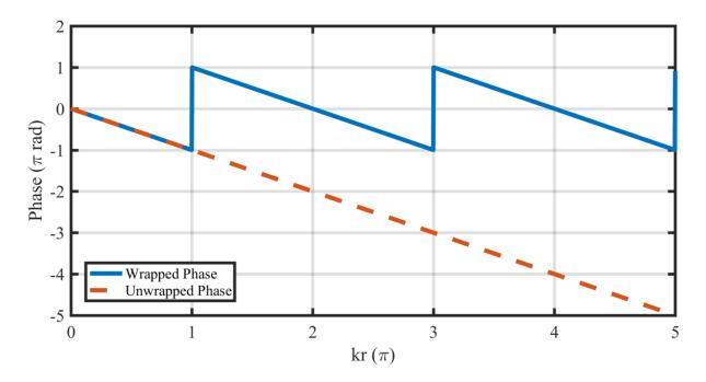
Figure 2.2. The phase for a plane wave as a function of kr for r=1m and zero initial phase. The wrapped phase has discontinuities at odd multiples of  $\pi$ . The unwrapped phase correctly subtracts  $2\pi$  to the wrapped phase in order to produce a continuous line.
