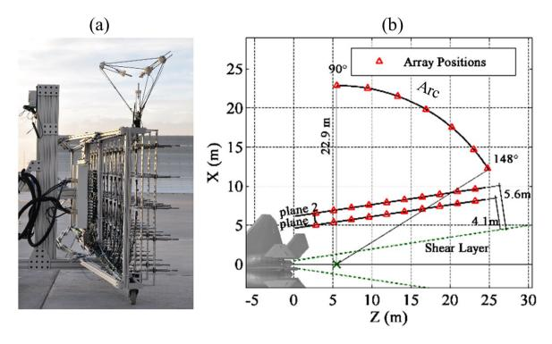
Figure 5.1. Experimental Setup. (a) Photograph of the intensity probe on top of the 90 microphone array. (b) Schematic of noise measurements of a tethered high-performance military aircraft. The red triangles indicate the positions of the 90 microphone array.
