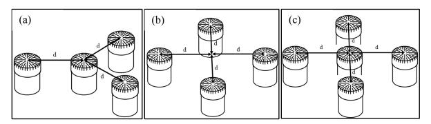
Figure 4.1. The three probe configurations: (a) equilateral triangle with a microphone at the center, (b) the orthogonal pair of microphones with no microphone at the center, and (c) the orthogonal pair of microphones with a microphone at the center.
