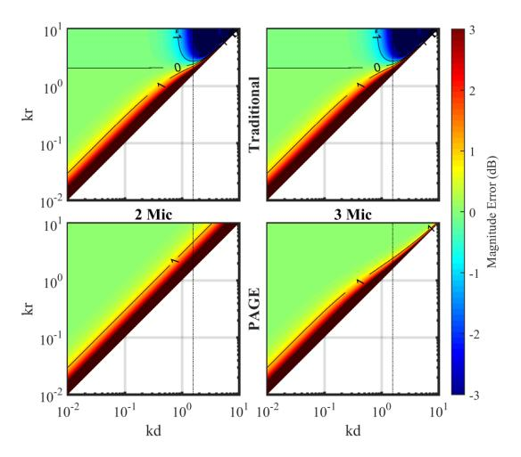
Figure 3.19. Relative error for kinetic energy density as a function of kd and kr. The black line indicates the spatial Nyquist limit. The PAGE method estimate with the three-microphone probe has less error at higher frequencies, but the two-microphone probe has a constant bias error. The traditional method's analysis is again frequency dependent and worsens near the Nyquist limit.
