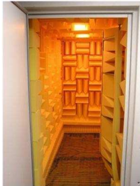
FIG. 3. Photograph of the anechoic chamber used with exposed foam wedges. The door to the chamber is open in this photograph.
