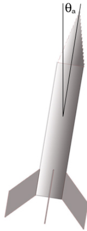
Figure 1. The angle between the vertical axis and the rocket's trajectory is the angle of attack.
