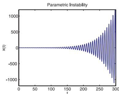
**Figure 10.2** Pumped swing instability.
