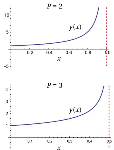
**Figure 2.1** The explosive growth function defined by Eq. 2.3 for two values of  $P$ .
