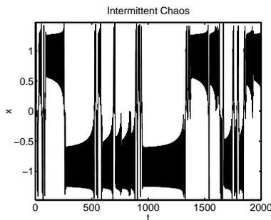
**Figure 12.2** Intermittent random bouncing between the two wells.
