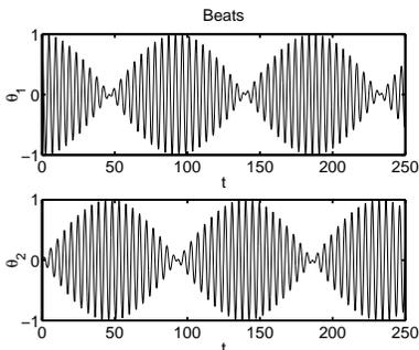
**Figure 13.1** Energy passes back and forth between  $\theta_1$  and  $\theta_2$  due to beating.
