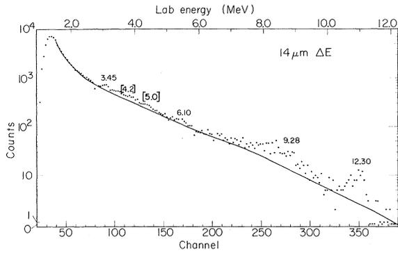
FIG. 2. Spectrum of delayed protons following the  $\beta$  decay of  ${}^9\text{C}$  as measured in a counter telescope employing a  $14\text{-}\mu\text{m}$   $\Delta E$  detector. Protons with laboratory energies above  $\sim 8.0$  MeV were not reliably detected in this telescope because of their small energy loss in this thin  $\Delta E$  detector. Energies in brackets denote possible peaks above the continuum.
