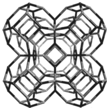
FIG. 2. The sodalite framework. Note how the \beta cage of Fig. 1 is used to construct a body-centered cubic lattice of cages.
