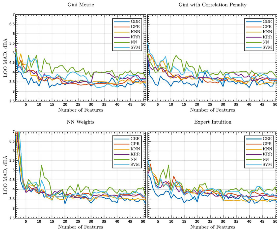
FIG. 1. (Color online) LOO MAD errors for the summer daytime A-weighted L_{50} as a function of the number of features. Model hyperparameters were tuned at 51, 40, 30, 20, 15, 10, 5, 4, 3, 2, and 1 feature(s).
