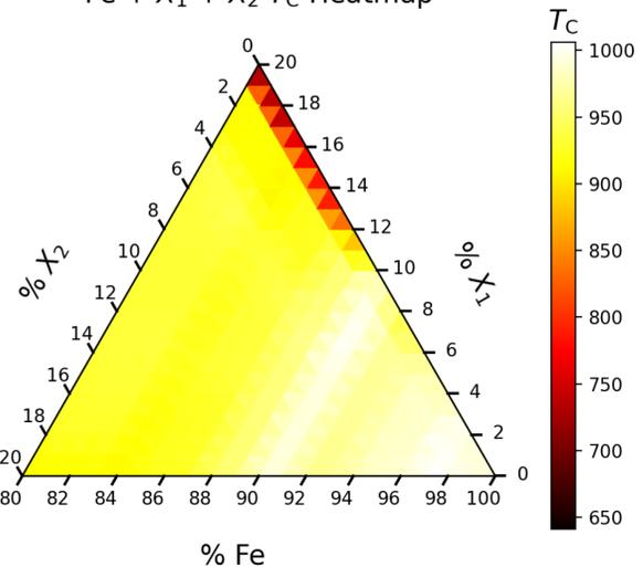
**FIG. 11.** Heat map showing the maximum predicted  $T_C$  of each combination of iron,  $X_1$  and  $X_2$  where  $X_1$  and  $X_2$  can be any element in materials with a  $T_C$  over 600 K found in DS1 and DS2 excluding cobalt and iron. Each compound is composed of a minimum of 80% iron.  $T_C$  is measured in Kelvins. Plot created using Python-Ternary.<sup>40</sup> (This plot should not be directly compared with Fig. 10 because of the difference in color scales.)
