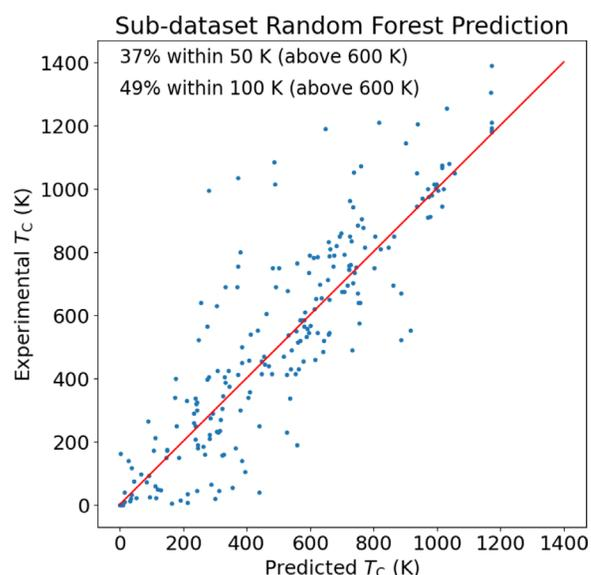
**FIG. 6.** Random-forest prediction with a balanced dataset. The Curie temperatures of the test data above 600 K were predicted with an accuracy of 37% of the data within 50 K and 49% within 100 K. The mean absolute error for those points was 141 K.
