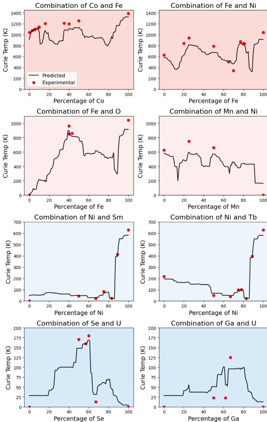
**FIG. 8.** Eight plots showing the Curie temperatures for eight different binary compounds. Horizontal rows share the same scale on the y axis. The black lines show the random-forest-predicted Curie temperatures across the entire composition range (step size: +1 at. %). The red dots are experimental data.
