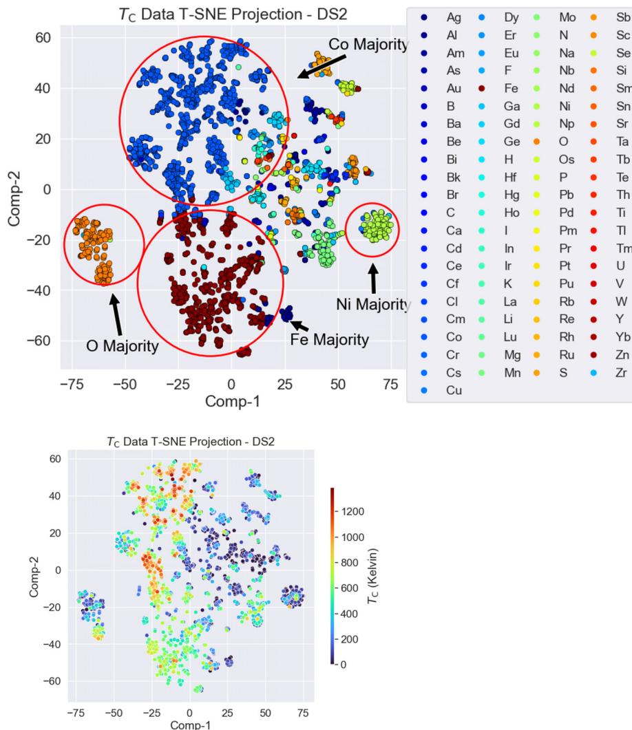
**FIG. 2.** (a) Experimental data (DS2) projected from the 85-dimensional feature space to two dimensions in a t-SNE<sup>34</sup> plot. Colors were assigned based on the majority element in each compound. (b) DS2 represented as a two-dimensional t-SNE plot. Colors were assigned based on the Curie temperature.
