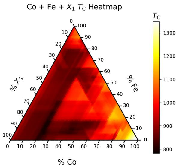
**FIG. 10.** Heat map showing the maximum predicted  $T_C$  of each combination of cobalt, iron, and  $X_1$ , where  $X_1$  can be any element in materials with a  $T_C$  over 600 K found in DS1 and DS2 (excluding cobalt and iron).  $T_C$  is measured in Kelvins. Plot created using Python-Ternary.<sup>40</sup>
