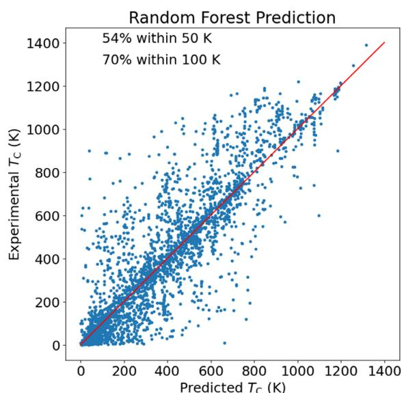
**FIG. 4.** Random-forest model trained on DS1 and validated with DS2. 54% of the  $T_C$  predictions for DS2 were within 50 K of the actual values and 70% were within 100 K. The mean absolute error was 90 K.
