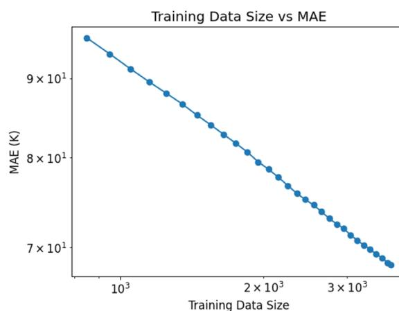
**FIG. 7.** MAE vs the amount of training data in a combined set of DS1 and DS2. For each iteration, the test data were a new random sample of 850 compounds while the training data were randomly sampled from the remaining data.
