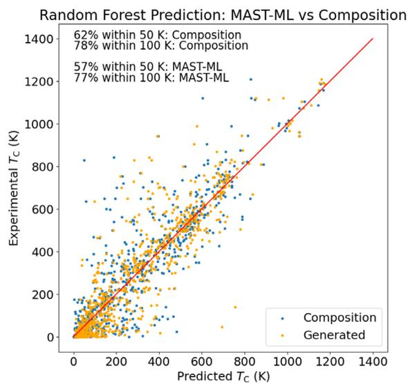
**FIG. 5.** Random-forest prediction using features based on the composition and 20 of the features generated by the MAST-ML<sup>38</sup> Python library. 62% of the  $T_C$  predictions for DS1 were within 50 K of the actual values, and 78% were within 100 K. The mean absolute error was 69 K. 57% of the  $T_C$  predictions for the MAST-ML data were within 50 K of the actual values, and 77% were within 100 K. The mean absolute error was 70 K.
