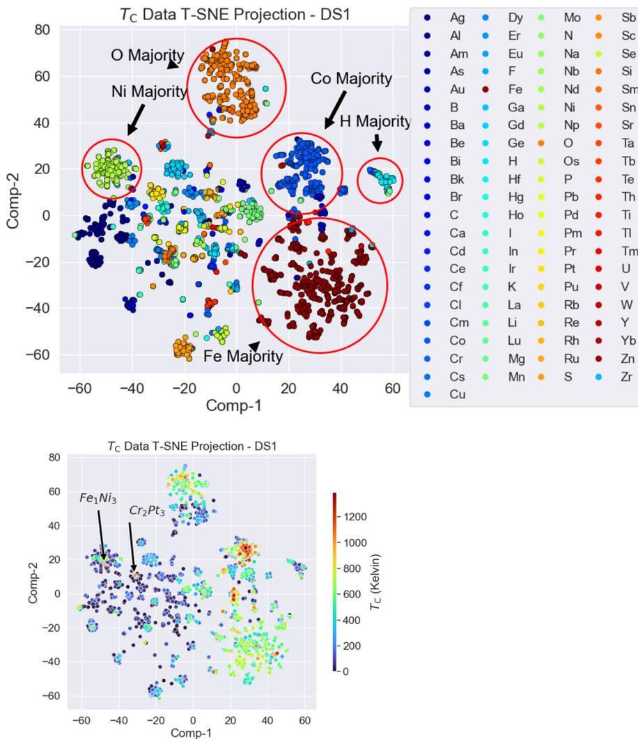
**FIG. 1.** (a) Experimental data (DS1) projected from the 85-dimensional feature space to two dimensions in a t-SNE<sup>34</sup> plot. Colors were assigned based on the majority element in each compound. (b) DS1 represented as a two-dimensional t-SNE plot. Colors were assigned based on the Curie temperature. Two compounds,  $Fe_1Ni_3$  and  $Cr_2Pt_3$ , have anomalously high Curie temperatures, relative to others in the same cluster.
