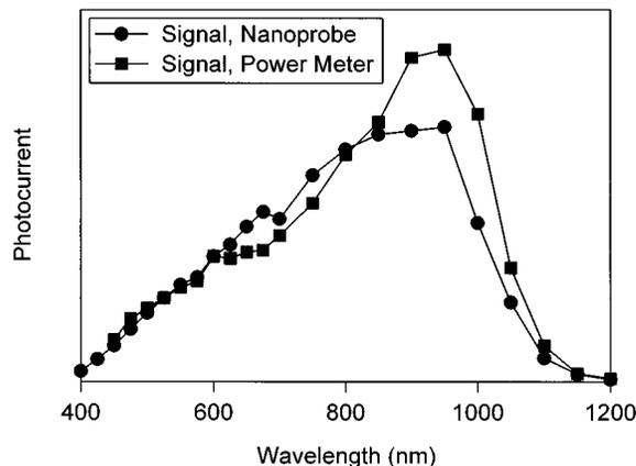
FIG. 4. The spectral response of the nanoprobe compared with a commercial photodetector. Both show a similar response.
