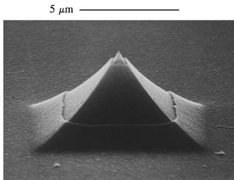
FIG. 2. A SEM image of the nanoprobe detector.
