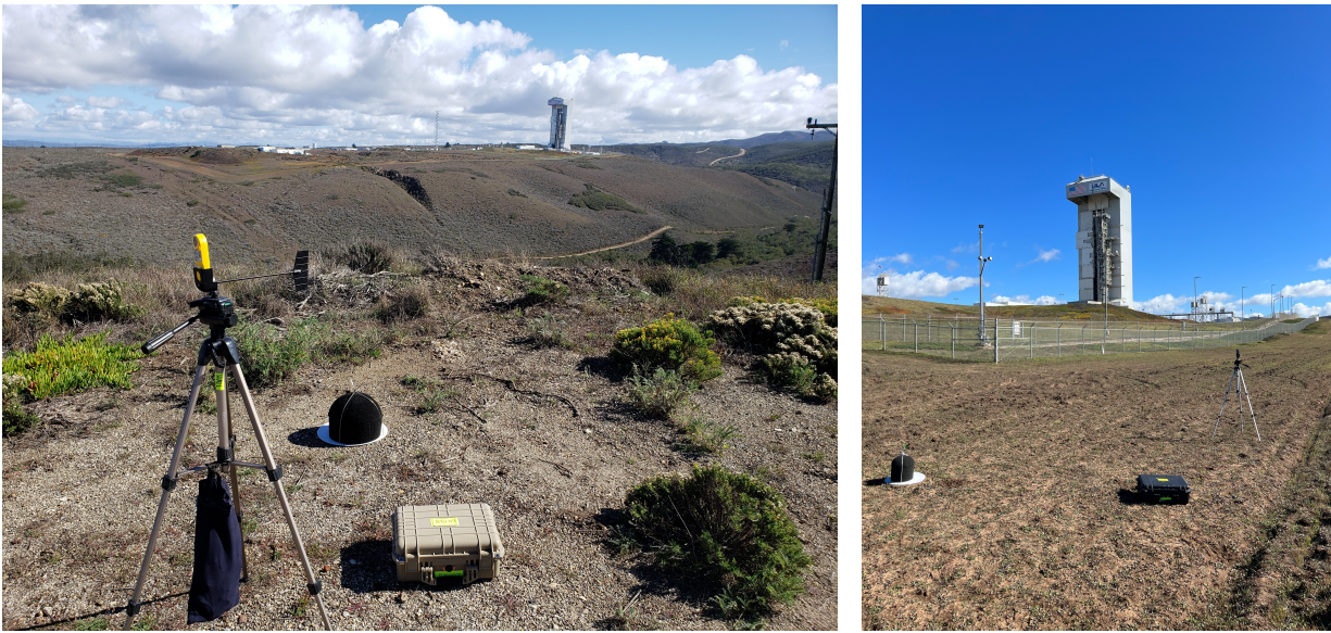
Figure 4. (Left) Station 7 at 1.1 km. (Right) Station 6 at 283 m. In both images, the launch facility Mobile Service Tower is visible, and within it is the rocket. Also visible in the foregrounds are the microphone ground plate/windscreen setups, instrumentation boxes, and weather stations.
