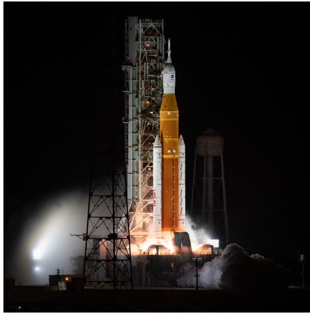
Figure 1. SLS Artemis-I ignition overpressure event (visible cloud at bottom left) during liftoff from LC-39B at Kennedy Space Center. Photo Credit: NASA.
