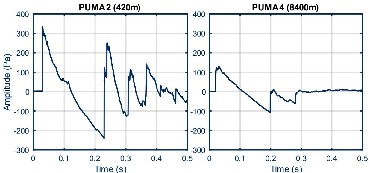
**Figure 5.** Sonic boom waveforms at PUMA 2 and PUMA 4 show that the sonic boom coalesces into three main shocks at distances farther from the pad.
