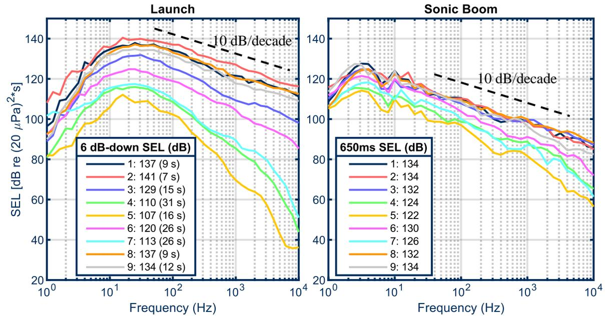
**Figure 6. One-third octave spectra and SEL for every PUMA microphone station for both the launch (trimmed to 6 dB-down points) and sonic boom.**
