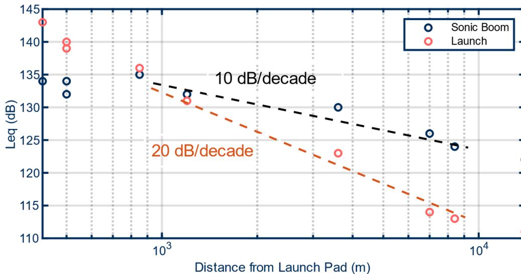
Figure 8. 1-second maximum equivalent level ( $Leq$ ) as a function of distance, showing the launch spreads spherically, and the sonic boom cylindrically.
