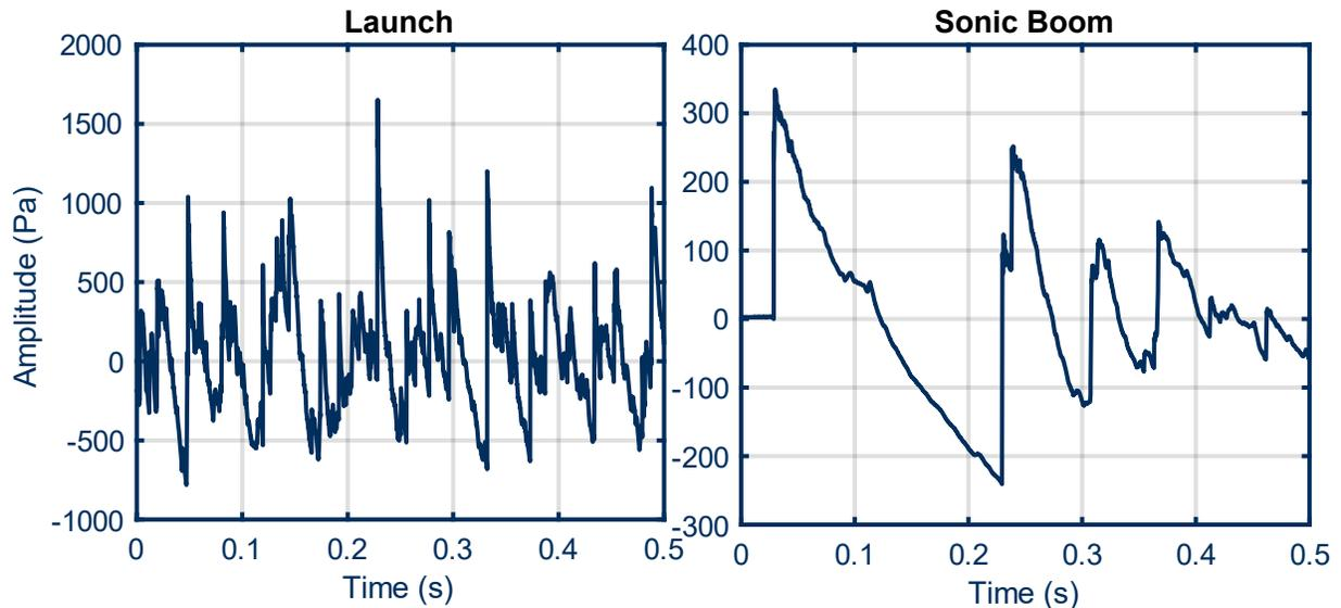
**Figure 4.** Waveform snippets of the launch (left) and sonic boom (right) from PUMA 2. Note the difference in the y-axis scale for the two plots.
