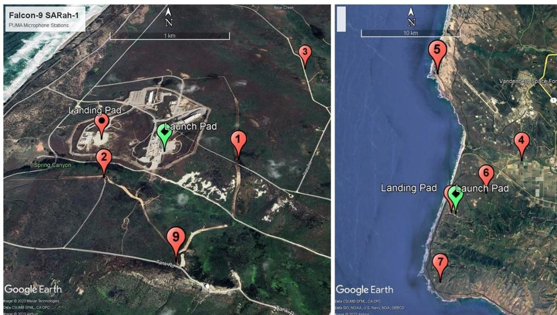
**Figure 2.** Left: Microphone stations (PUMAs) near the launch pad (green pin) and landing pad (red pin). Note: PUMAs 1 and 8 were at the same location. Right: Four PUMAs farther from the launch pad.
