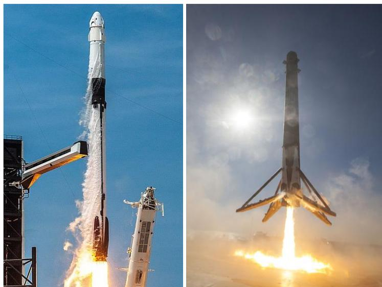
**Figure 1. Left: Photo of the Falcon-9 launch for the Demo-2 mission. Right: Falcon-9's first stage lands successfully following a launch. Image credit: NASA.**
