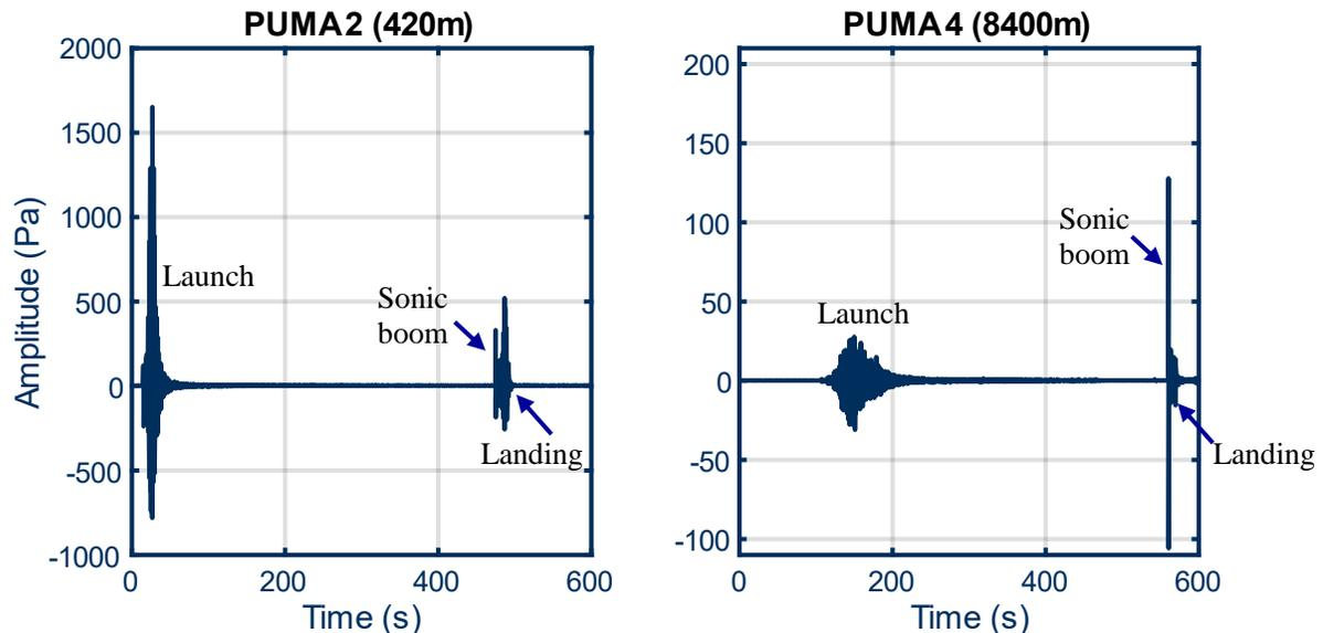
*Figure 3. Full waveforms for PUMA microphone stations 2 and 4, showing the launch, sonic boom, and landing noise. Note the difference in the y-axis scale for the two waveforms.*
