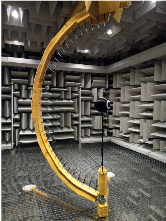
FIG. 9. (Color online) Directivity measurement system assessing the radiation of a spherical loudspeaker positioned at its center. The white disk controls the aperture size.
