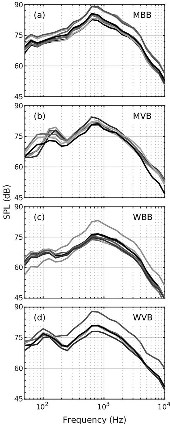
FIG. 4. The mean 1/3-octave spectrum for each game, separated by sport type.
