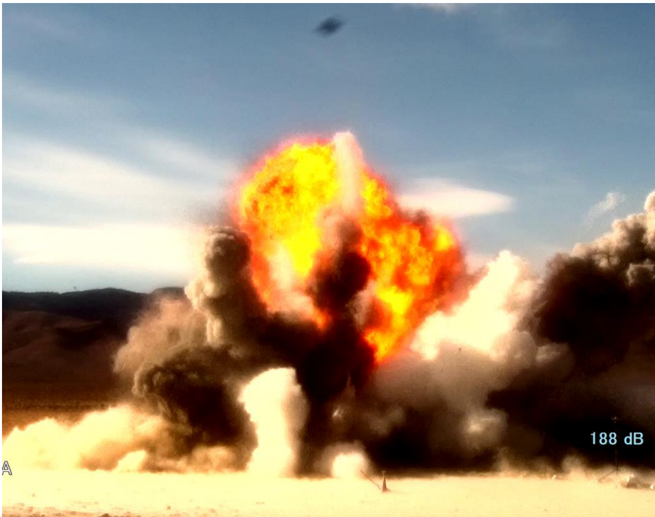
Figure 1. Image of 02/16/21 120 lb. C4 shot with measured peak level labeled (located at 19m from blast).
