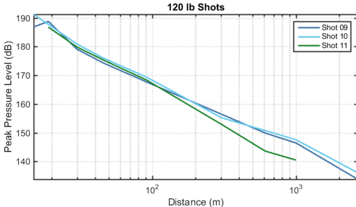
Figure 9. Peak pressure level decay for 120 lb. C4 explosions as a function of distance
