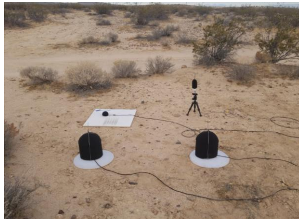
Figure 7. Comparative station at CarpetDIEM I. (Top Left) a Ground-Board configuration. (Top Right) An Elevated configuration, with the microphone raised 18 inches (46 cm) above the ground. (Bottom) Two COUGAR configurations with different microphones. The Ground-Board, Elevated, and COUGAR configurations compared in this paper all use a PCB 378A07 microphone. This station is referred to as PUMA 1 in Durrant et al. (2022).
