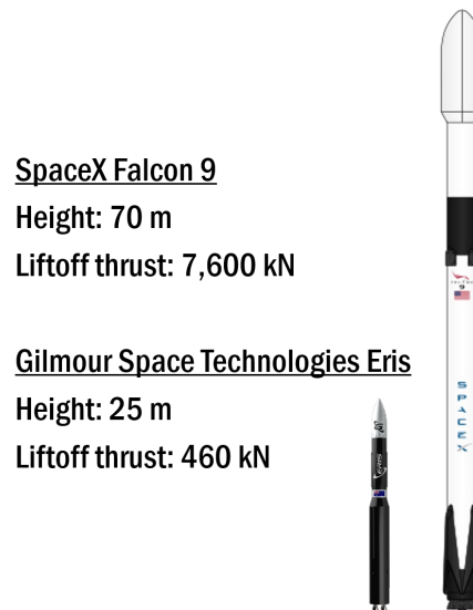
Figure 3. A comparison between the Gilmour Eris and the SpaceX Falcon 9 rockets.
