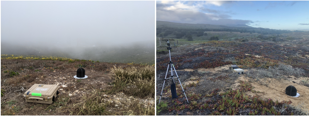
Figure 2: Example measurement station consisting of an inverted microphone placed over a hard plastic ground plate and covered by a dome windscreen, with all other electronics placed inside a weather-resistant case. Some locations also included small weather stations mounted on tripods.
