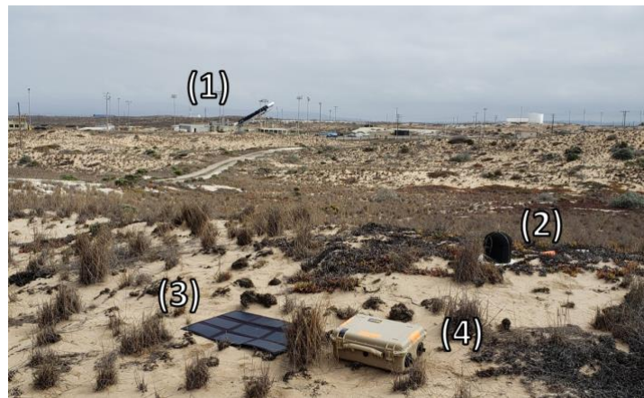
Figure 3. Data collection equipment at Station 9 with Alpha in background. (1) Firefly Alpha, (2) windscreen and ground plate housing microphone, (3) solar panel, (4) weatherproof case.
