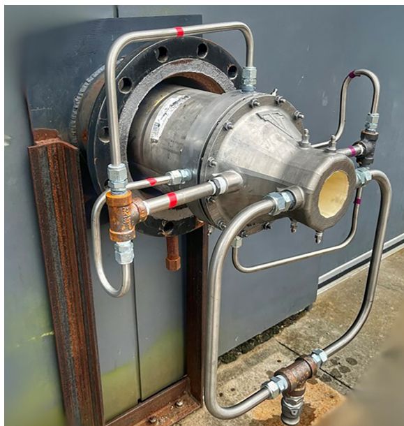
FIG. 3. Scaled-down F-404 nozzle with cooling water lines.
