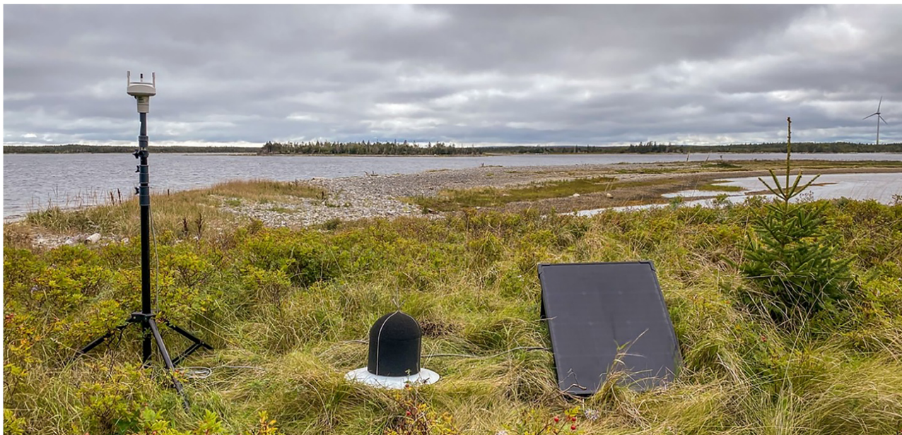
FIG. 3. Photograph of BRRC's soundscape measurement setup.
