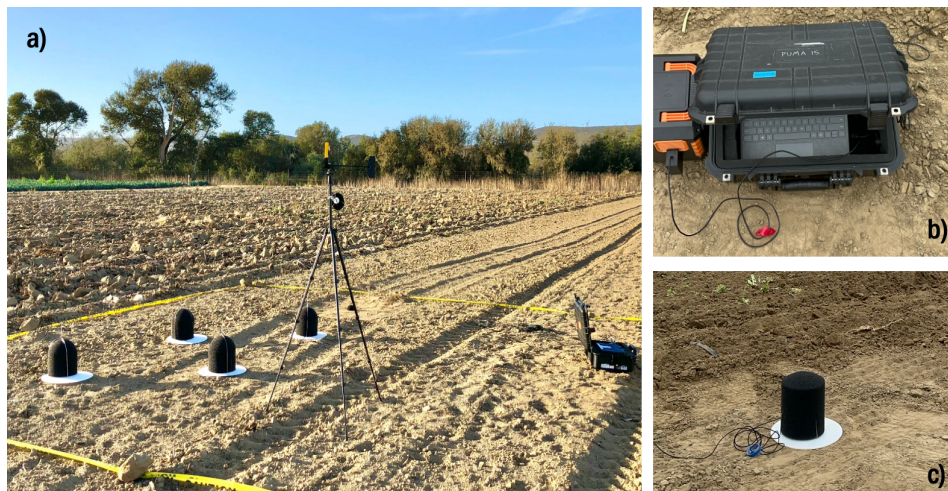
Figure 2. a) An example measurement set-up. b) PUMA computer and DAQ system. c) COUGAR windscreens and microphone deployment.
