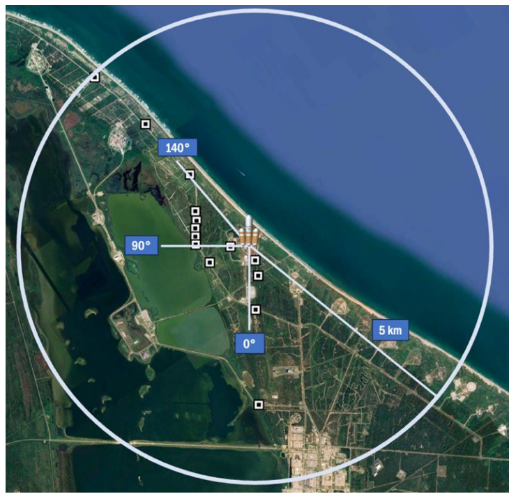
Figure 6. Overview of measurement sites during NROL-70. Stations ranged from 150 m to 5 km from the launch pad. The 0^\circ , 90^\circ , and 140^\circ lines relative to the rocket are noted. (Google Earth Pro, Image © 2026 Google).
