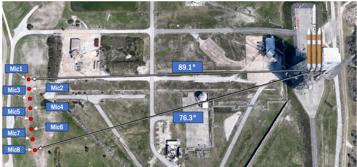
Figure 5. Overview of measurement set-up at site 16. Microphones span an aperture of 12.8^\circ . General rocket location and orientation is noted (not to scale). (Google Earth Pro, Image © 2026 Google).
