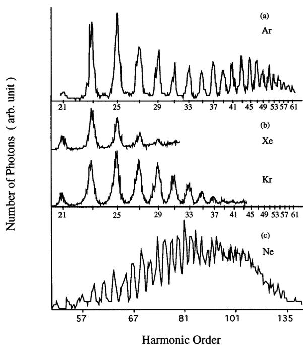
FIG. 1. Harmonic spectra generated in (a)  $\sim 5$  Torr of Ar, and (b) 2 Torr of Kr and Xe, with peak laser intensity  $5 \times 10^{14} \text{ W/cm}^2$ . (c) Harmonic spectra generated in  $\sim 10$  Torr of Ne with peak laser intensity  $2 \times 10^{15} \text{ W/cm}^2$ . The relative intensities of (a)–(c) should not be compared directly.
