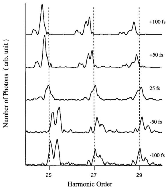
FIG. 3. Theoretical predictions for the harmonic spectra generated for various excitation laser chirp for fixed intensity and bandwidth.
