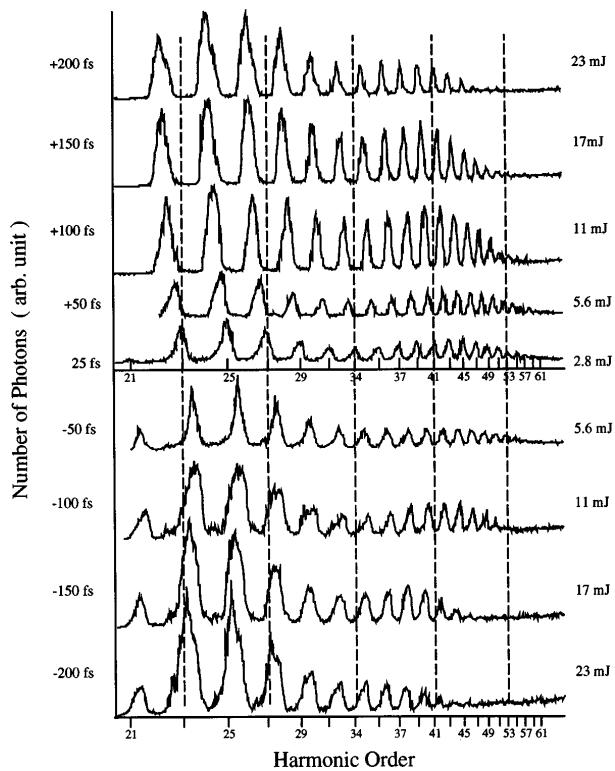
FIG. 2. Harmonic spectra generated in 5 Torr of argon for fixed peak laser intensity of  $5 \times 10^{14} \text{ W/cm}^2$  and for various laser pulse chirps.
