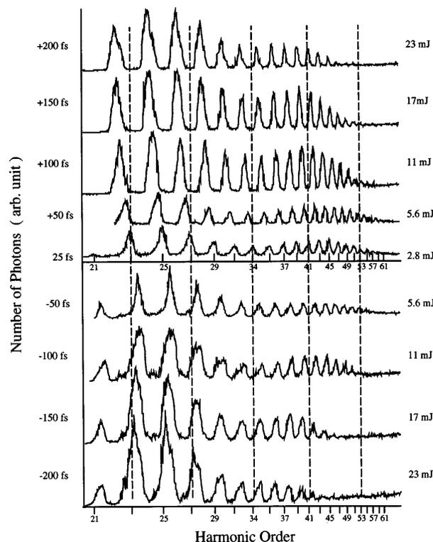
FIG. 2. Harmonic spectra generated in 5 Torr of argon for fixed peak laser intensity of  $5 \times 10^{14}$  W/cm<sup>2</sup> and for various laser pulse chirps.
