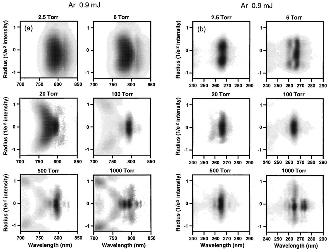
Fig. 4. (a) Fundamental and (b) third-harmonic spectra as functions of beam radial position for a pulse energy of 0.9 mJ focused in various pressures of argon. Position is expressed in units of  $1/e^2$ -intensity radius of the beam when the gas cell is evacuated. The brightness of the images should not be compared from frame to frame.
