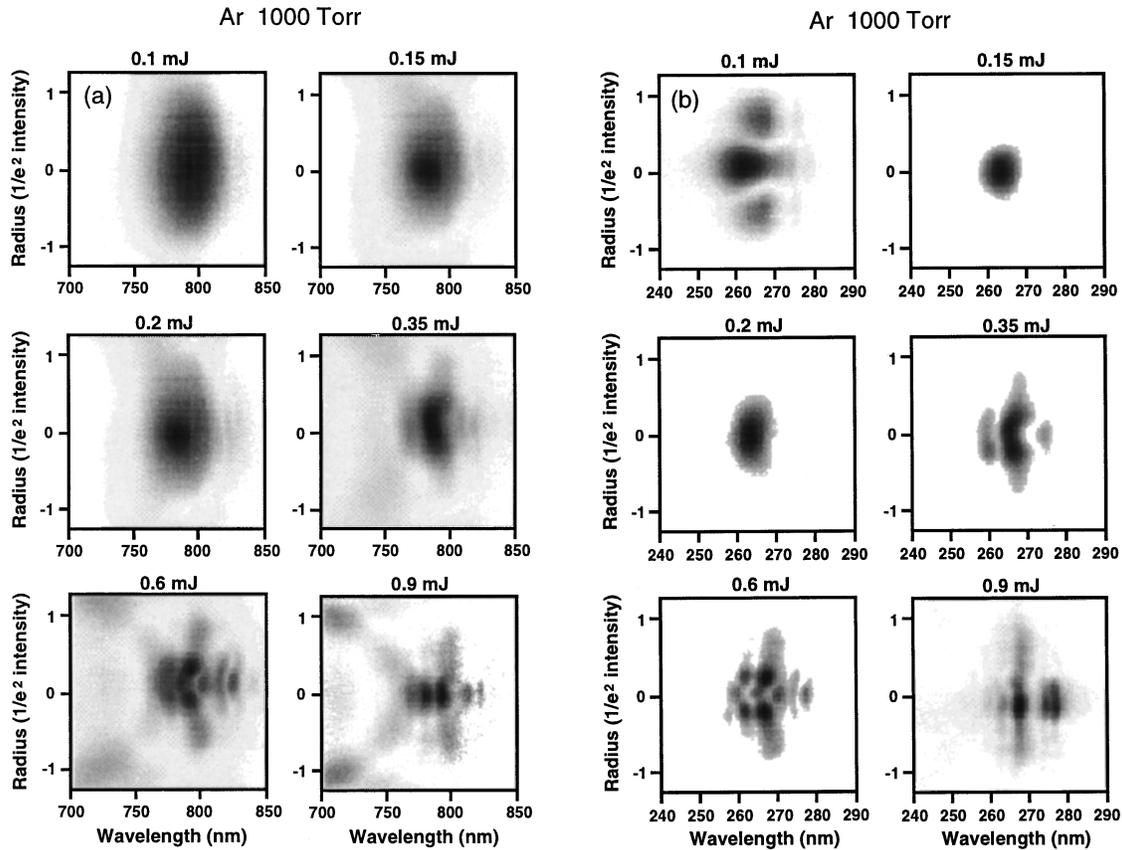
Fig. 3. (a) Fundamental and (b) third-harmonic spectra as functions of beam radial position for various pulse energies focused in 1000 Torr of argon. Position is expressed in units of  $1/e^2$ -intensity radius of the beam when the gas cell is evacuated. The brightness of the images should not be compared from frame to frame.
