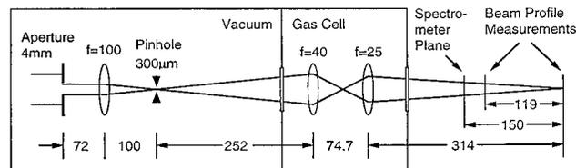
Fig. 1. Experimental setup: The laser beam is apertured and spatially filtered before it is focused inside a gas cell. The emerging light is collected and imaged to a far distance. A spectrometer intersects the beam for spectral analysis as a function of radial position. Near-normal-incidence curved mirrors were used rather than the three lenses depicted for convenience. The dimensions are given in centimeters.
