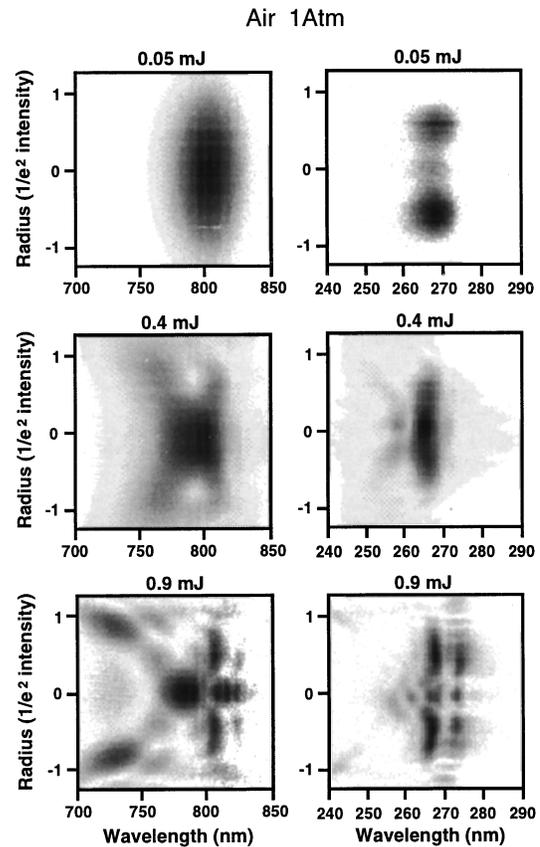
Fig. 6. Fundamental (left column) and third-harmonic (right column) spectra as functions of beam radial position for various pulse energies focused in 1 atm of air. Position is expressed in units of  $1/e^2$ -intensity radius of the beam when the gas cell is evacuated. The brightness of the images should not be compared from frame to frame.
