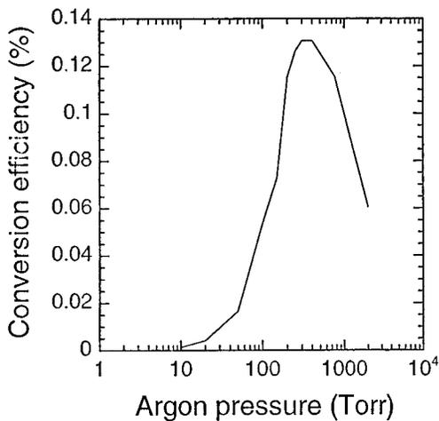
Fig. 5. Conversion efficiency of the third harmonic as a function of argon pressure.
