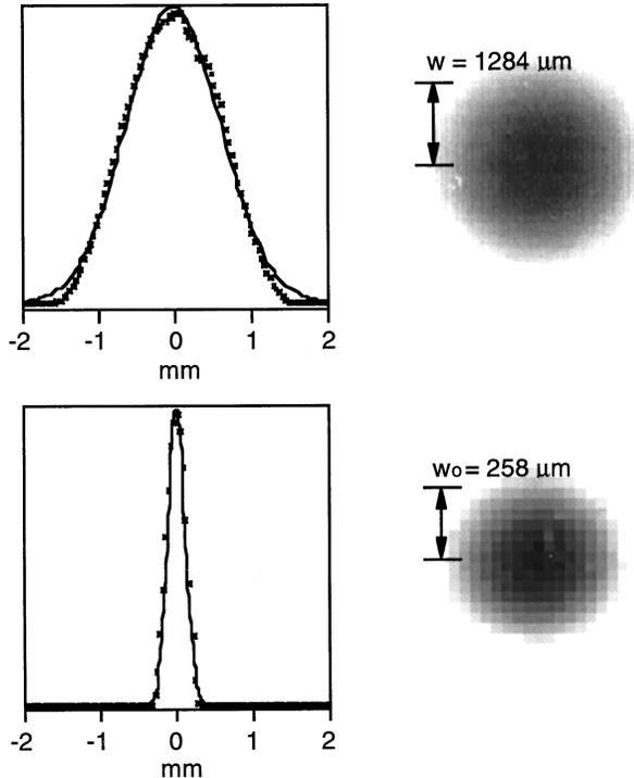
Fig. 2. Radial profiles and corresponding images of the laser beam profile. As indicated in Fig. 1, the beam profile was measured to be 119 cm before (upper) and at the imaged focus (lower). The upper contour data is shown together with a best-fit Gaussian curve. This curve is used to calculate the diffraction-limited curve shown together with the data taken at the imaged focus (lower).
