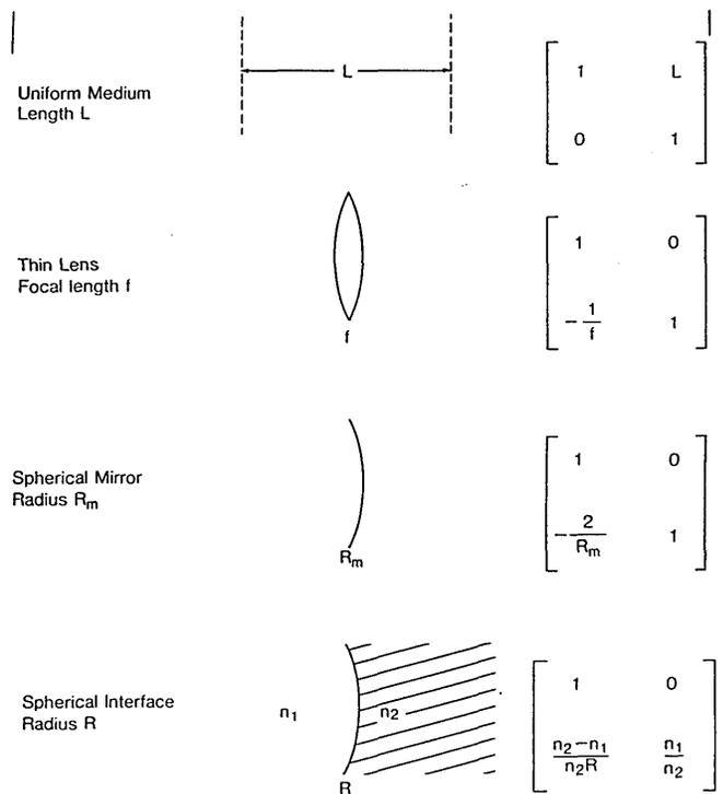
Fig. 1. ABCD matrices for a few simple optical elements. Gaussian beam is assumed to be incident from the left.
