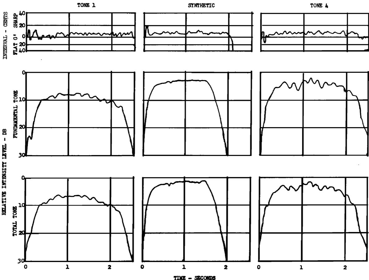
Fig. 2. Frequency and intensity level vs time for violin G'.
