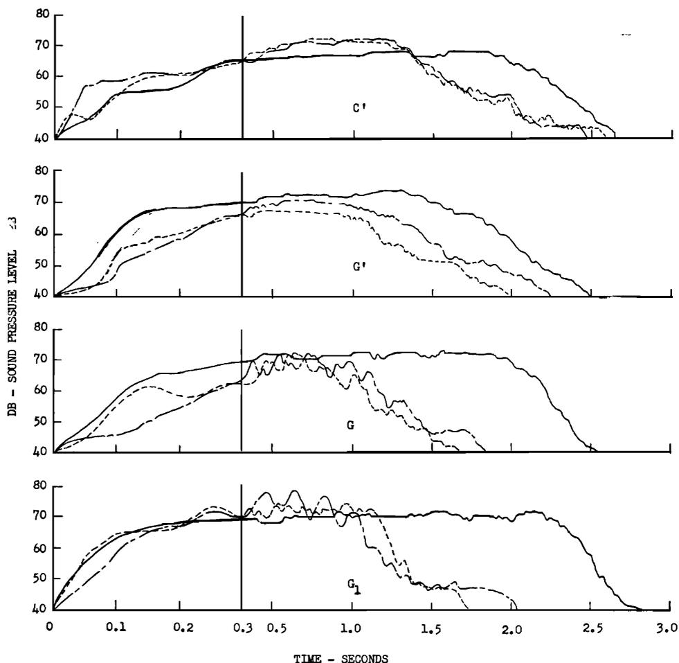
FIG. 12. Sound-pressure level vs time for viola tones.
