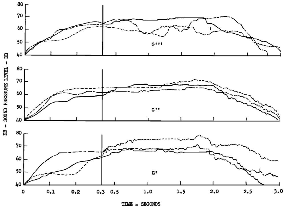
FIG. 14. Sound-pressure level vs time for bass-viol tones. - - - - Real tone. ——— Real tone. ——— Synthetic tone.
