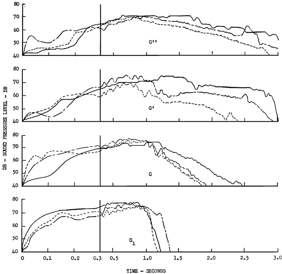
FIG. 13. Sound-pressure level vs time for 'cello tones. - - - - Real tone. - - - - Real tone. ——— Synthetic tone.
