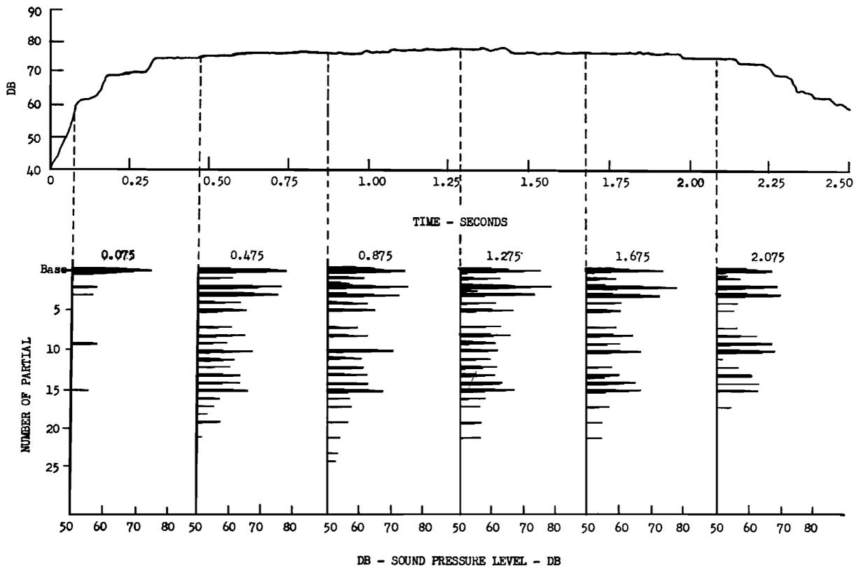
FIG. 7. Sonogram for G', tone 4. The over-all sound-pressure level is plotted at the top.
