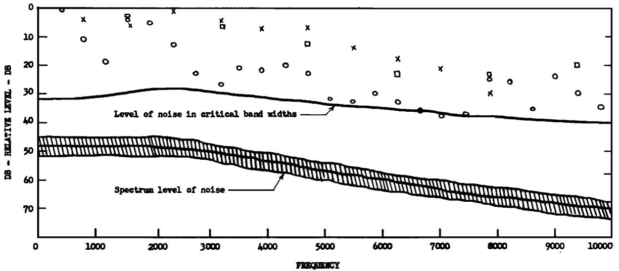
FIG. 6. Noise levels vs frequency for violin playing. Circles for partials of G, crosses for G<sub>1</sub>, squares for G<sub>2</sub>.
