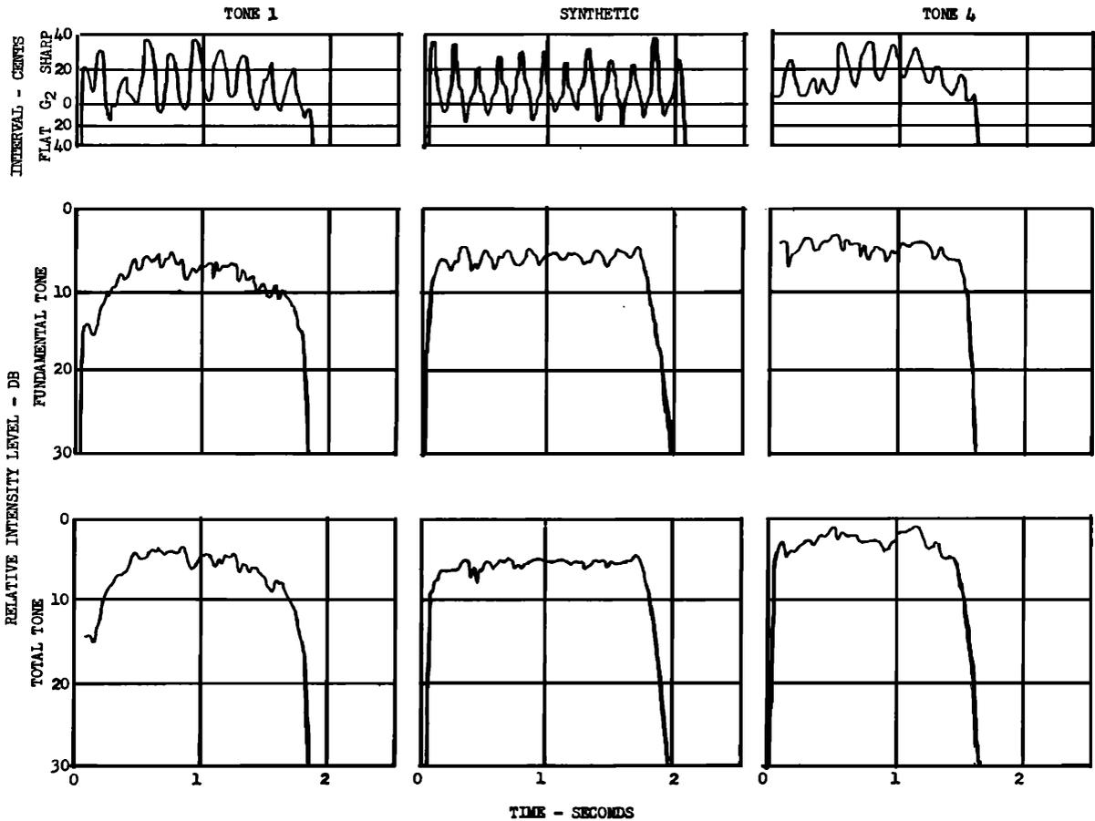
FIG. 5. Frequency and intensity level vs time for violin G<sub>2</sub>.
