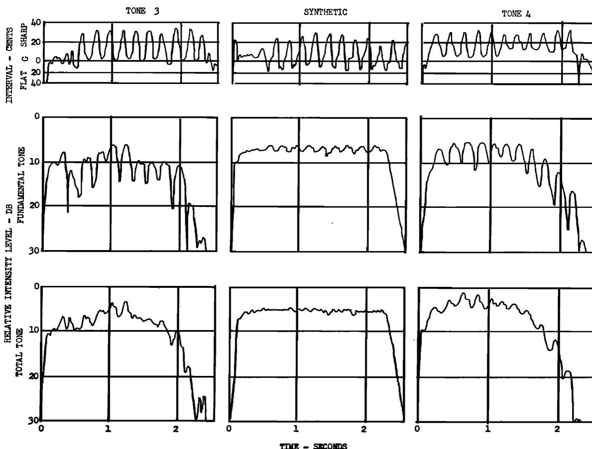
FIG. 3. Frequency and intensity level vs time for violin G.
