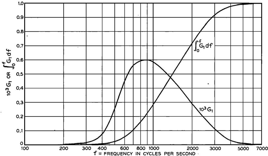
FIG. 9. The functions  $G_1$  and  $\int_0^f G_1 df$ .  $G_1$  is the frequency weighting factor for loudness, when speech is at the threshold of audibility. (See also Fig. 50 and Table VIII.)
