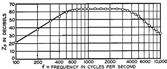
FIG. 11. Level  $Z_F$  of each critical band of undistorted speech in decibels above threshold, when the speech is at the optimum level for interpretation.
