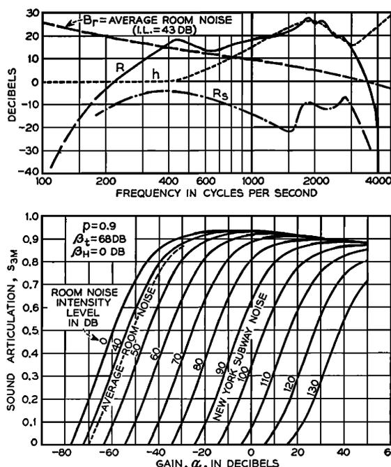
FIG. 48. Calculated articulation vs. gain for commercial system with room noise at listener's location.  $R$  = Response of system.  $B_r$  = Acoustic noise spectrum level.  $h$  = Attenuation of noise going under earphone cap to the ear.  $R_s$  = Sidetone response.  $I.L.$  = Total intensity level.
