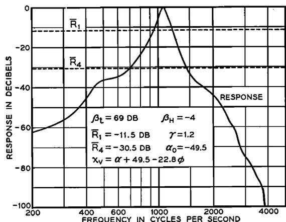
FIG. 10. Response of resonant system II-RN-1060, with weighted averages  $\bar{R}_1$  and  $\bar{R}_4$  and values of  $\gamma$ ,  $\alpha_0$  and  $\alpha_T$ .
