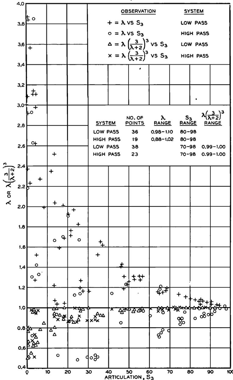
FIG. 2. Observed values of  $\lambda$  and  $\lambda(3/\lambda+2)^3$  vs. syllable articulation  $S_3$  for filter systems.
