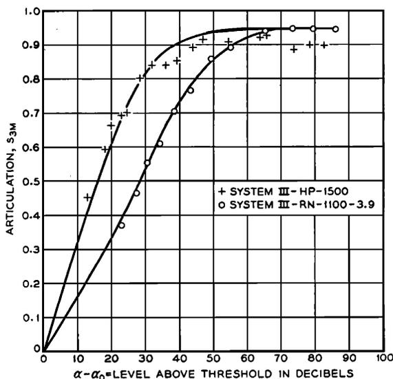
FIG. 12. Articulation vs. level of received speech above threshold, for a resonant system and a filter system having approximately equal maxima of articulation.
