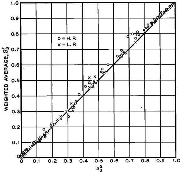
FIG. 6. Weighted average syllable articulation  $S_3'$  vs. cube of speech sound articulation  $s_3^3$  for filter systems.
