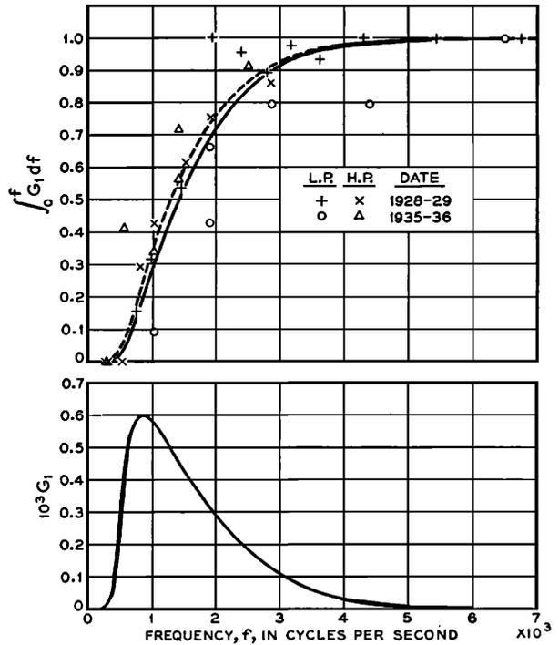
FIG. 50. Derivation of  $\int_0^f G_1 df$  and  $G_1$  from filtered speech thresholds. (See also Fig. 9 and Table VIII.) The discrete points in the upper plot show values of  $\int_0^f G_1 df$  vs.  $f_c$  derived in Table XXIX from observed thresholds.
