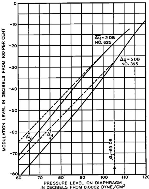
FIG. 20. Output vs. input characteristics of No. 395 and No. 625 carbon type microphones tested in a constant sound field at frequency 1000 c.p.s.
