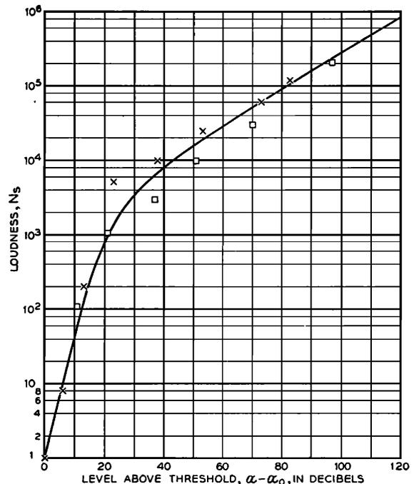
FIG. 52. Loudness of undistorted speech vs. level above threshold. Points observed, curve drawn to represent both sets of data.
