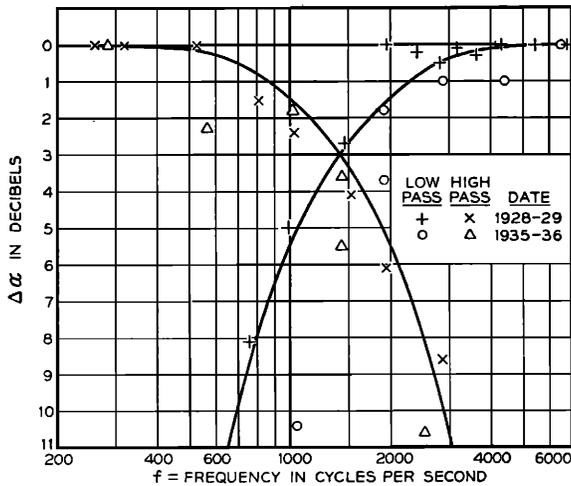
FIG. 51. Gain change  $\Delta\alpha$  required for speech to remain at threshold when cut-off frequency is changed from 0 or  $\infty$  to  $f$ . Points observed, curves calculated. Values of  $\Delta\alpha$  are zero or positive but are plotted increasing downward.
