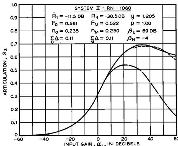
FIG. 19. Calculated articulation vs. gain for three conditions in regard to overload.
