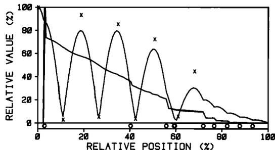
FIG. 4. Calculated pressure and power distributions in flute bore when fingered for  $A_6$  with open  $D\#$  key. Resonance frequency was 1780 Hz. Circles mark positions of open holes. Experimental values are shown by crosses.
