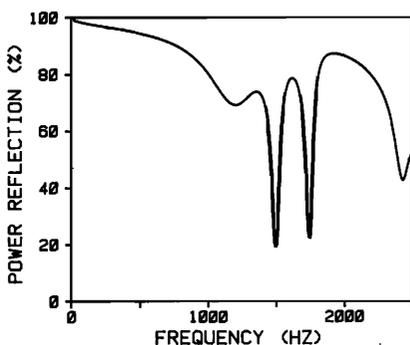
FIG. 7. Calculated power reflection coefficient for closed D# key fingering of  $A_6$ .
