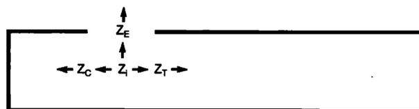
FIG. 2. Schematic of embouchure hole region of flute showing embouchure hole impedance  $Z_E$ , cork cavity impedance  $Z_C$ , and tube impedance,  $Z_T$ .  $Z_i$  is the impedance seen at the inside "end" of the embouchure hole.
