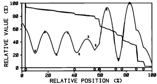
FIG. 8. Calculated pressure and power distributions in flute bore when fingered for  $A_6$  with closed D# key. Calculation was for a frequency of 1740 Hz near a minimum in the power reflection curve.
