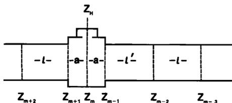
FIG. 1. Approximation of flute bore with contiguous cylindrical sections. Maximum section length is  $l$ ; a shortened section length  $l'$  precedes the closed tone hole. The section on either side of the tone hole center has a length equal to the hole radius  $a$ . The bore is enlarged and a small volume is placed in parallel with the bore to represent the effects of a closed tone hole.
