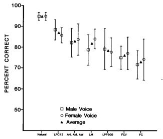
FIG. 3. Diagnostic Rhyme Test (DRT) intelligibility scores for various versions of speech and untransposed speech codes.
