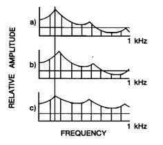
FIG. 2. Spectral effects of biasing and equalization using idealized spectra of AMT code (all-harmonic, modified-fundamental scaling, frequency lowered) (a) AMT, (b) AMTB, biased by 100 Hz, and (c) AMTL linear equalization. (Lines drawn on the graphs are references for comparison.)
