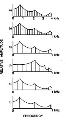
FIG. 1. Idealized spectra of the synthesized speech codes. (a) Original speech. (b) AH—all harmonic; fundamental scaled with spectrum. (c) AM—all harmonic, modified fundamental scaling. (d) AW—all harmonic; warped spectrum. (e) LM—largest harmonic. (f) FC—formant code. Note 4-kHz bandwidth in (a) but only 1 kHz in all others.
