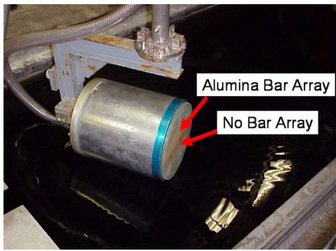
FIG. 5. (Color online) Photograph of the alumina bar array module used in experiments.
