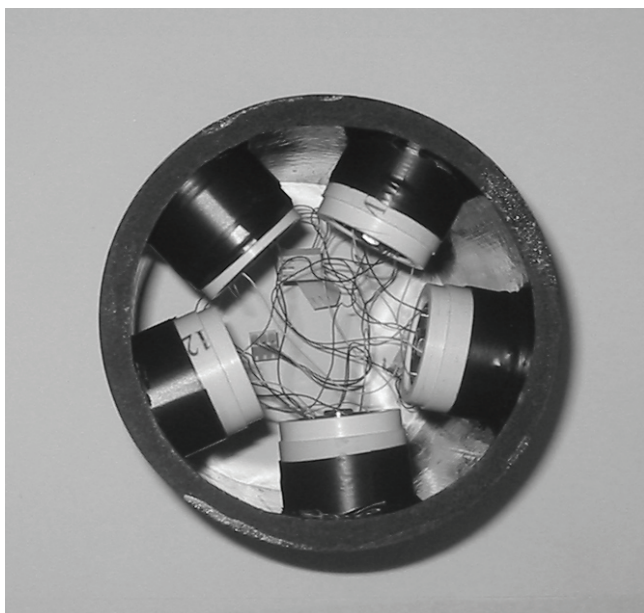
Fig. 5. Placement for five PCB 1 inch diameter microphones
