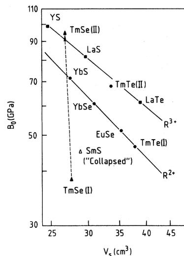
FIG. 4. Anderson-Nafe plots for rare-earth monochalcogenides. The lines  $R^{2+}$  and  $R^{3+}$  correspond, respectively, to the 2+ and 3+ valence state of the rare earth.
