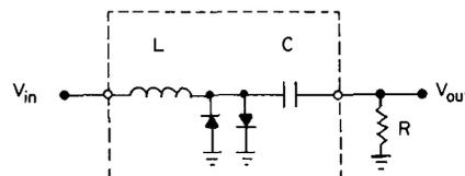
FIG. 1. Tuned limiter.  $L$  and  $C$  are series tuned to the NMR frequency.  $R$  represents the resistive load of the rf amplifier input.
