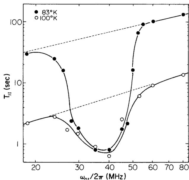
FIG. 7. Effect of Zeeman-quadrupole cross relaxation on  $T_{1I}$ .
