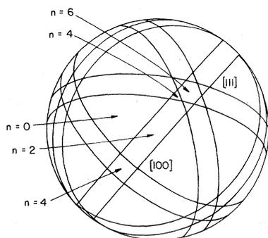
FIG. 2. Directions of  $\vec{\nabla}K$  which satisfy Eq. (6) for the twelve nearest neighbors in a face-centered-cubic lattice. The six bands are regions where two neighbors satisfy Eq. (6) simultaneously. Intersections of these bands give rise to regions where four and six neighbors satisfy Eq. (6) simultaneously. This figure is plotted for  $|\vec{\nabla}K| a\omega_0 / \omega_1 = 10$ .
