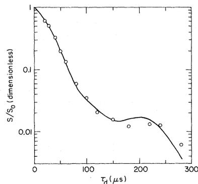
FIG. 7. Spin-echo amplitude  $S/S_0$  at  $H_0/\nu_0=1.138$  kG/MHz,  $\nu_0=74$  MHz, and  $T=77$  K. Solid line is the best fit to Eq. (10). See Table I.
