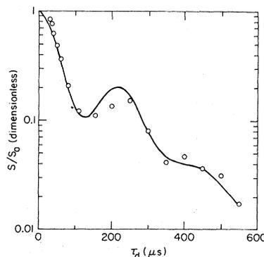
FIG. 9. Spin-echo amplitude  $S/S_0$  at  $H_0/\nu_0=1.138$  kG/MHz,  $\nu_0=8.4$  MHz, and  $T=4.2$  K. Solid line is the best fit to Eq. (10). See Table I.
