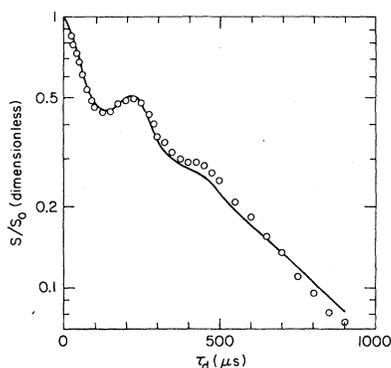
FIG. 8. Spin-echo amplitude  $S/S_0$  at  $H_0/\nu_0=1.117$  kG/MHz,  $\nu_0=74$  MHz, and  $T=4.2$  K. Solid line is the best fit to Eq. (10). See Table I.
