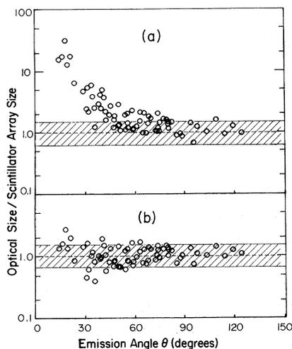
FIG. 4. Ratios of sizes obtained from the optical data to sizes measured by the Volcano Ranch array using (a) computed scintillation light only and (b) estimated light from all sources. Data are plotted for each phototube in all fifteen reconstructed showers. The shaded bands display the uncertainty due to systematic effects in both size measurements.
