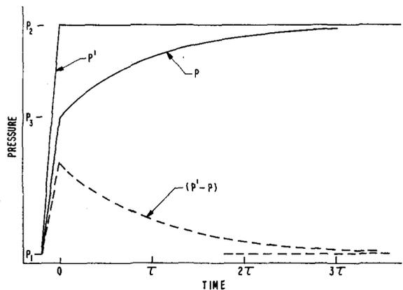
FIG. 3. Measurable pressure variations associated with an idealized viscosity determination using a constant pressure  $P'$  following a rapid linear increase.
