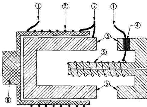
FIG. 4. Cross section of cylindrical viscometer showing details of construction. (a) Copper lead wires to extend out of capsule; (2) outside manganin gauge,  $M_0$ ; (3) inside manganin gauge,  $M_i$ ; (4) epoxy electrical feedthrough; (5) surfaces to be brazed to seal viscometer; (6) Teflon insulating sheath.
