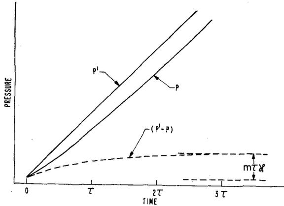
FIG. 2. Measurable pressure variations associated with an idealized viscosity determination using a linear increase of pressure  $P'$  with time.
