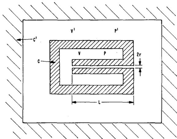
FIG. 1. Diagrammatic cross section of cylindrical viscometer giving nomenclature for mathematical derivations.
