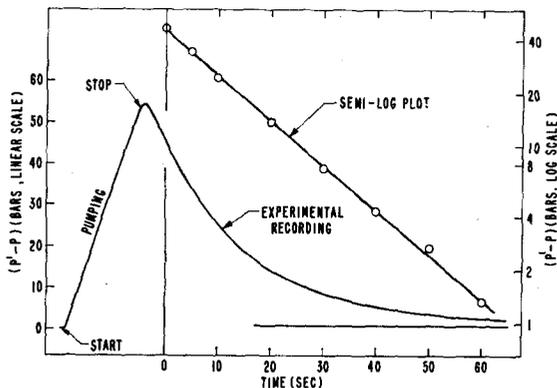
FIG. 6. Typical recorder trace of  $(P' - P)$  pressure differences as a function of time and corresponding semilog plot to illustrate exponential variation. Points were simply taken from recording.
