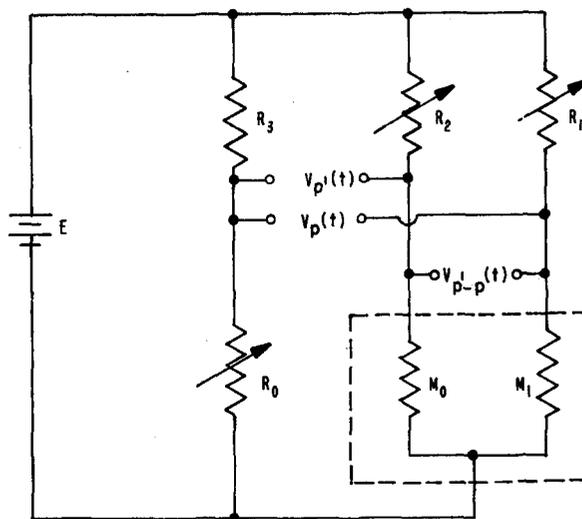
FIG. 5. Parallel Wheatstone-bridge circuit used for recording pressure changes detected by manganin gauges.
