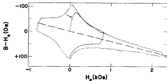
FIG. 5. Dc tube magnetization curve at 13.85°K. The zero magnetization axis (dashed line) is tilted due to a 2.8% mismatch in the two sensing coils. The final part of the curve does not close completely because of drifts from residual thermal emf's. (The slope of the Meissner region is not 45° because of the different scale factors used for the  $x$  and  $y$  axes and because of the demagnetizing factor.)
