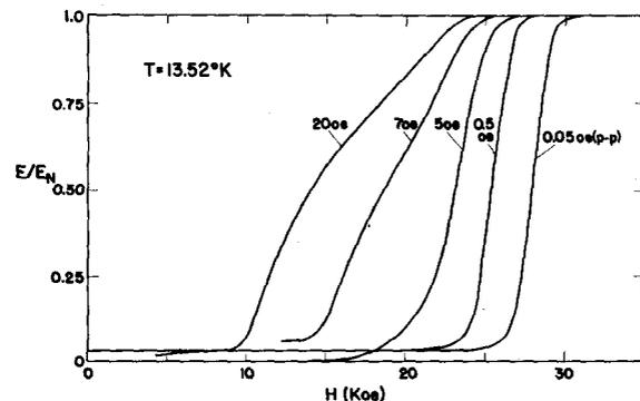
FIG. 2. Transitions in dc magnetic field for various ac levels at  $13.52^\circ\text{K}$ . Normalized ac signal from pickup coil,  $E/E_N$ , where  $E_N$  is the normal state limiting value of the ac signal  $E$  plotted as a function of the dc field  $H$  for various indicated values of the alternating field intensity.
