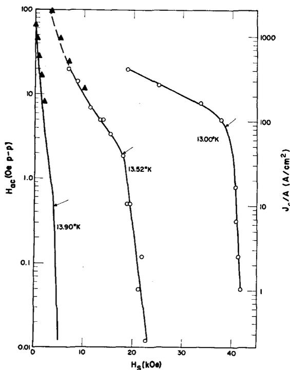
FIG. 3. Critical current curves. The maximum permissible alternating field intensity  $H_{ac}$  as a function of the lower threshold field  $H_S$  at various temperatures. Corresponding induced supercurrent densities are given by scale on right. The arrows indicate the position of the knee  $H_K$ . The solid triangles are taken from the dc measurements.
