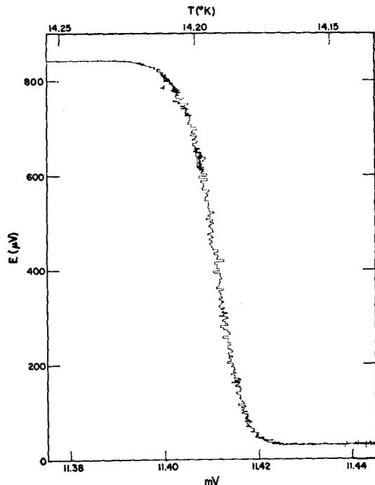
FIG. 1. Zero field transition at 100 kHz, 0.05 Oe p-p. Ac signal  $E$  from pickup coil as a function of carbon resistor thermometer voltage, mV, at a fixed measuring current of  $103.5 \mu\text{A}$  (lower scale) and corresponding temperature  $T$  (upper scale). Steps are caused by 1-sec sampling period of digital voltmeter used for carbon thermometer readout.
