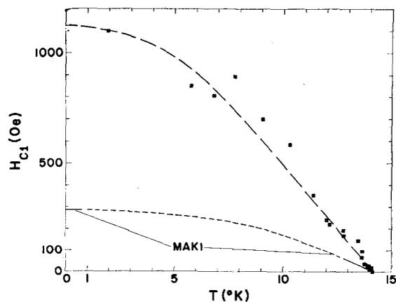
FIG. 6. Temperature variation of lower critical field. ■ Experimentally from break of Meissner line. — Calculated from Maki's relations using the experimental value of  $\kappa$ .
