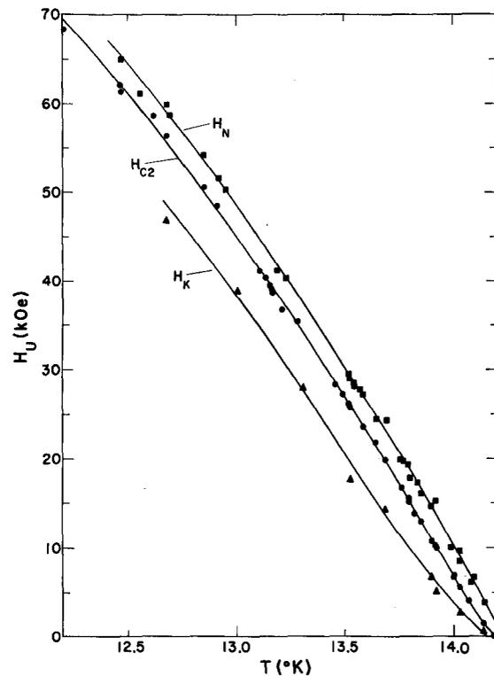
FIG. 4. Temperature variation of various upper critical fields.  $H_K$  represents the field at the knee of the critical current curves in Fig. 3.  $H_{c2}$  represents the midpoint of the "standard" 100-kHz, 0.05-Oe p-p transition.  $H_N$  represents the first indication of superconductivity.
