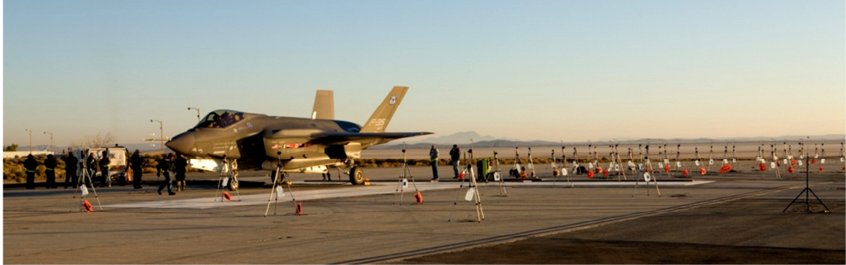
Figure 1. Tied-down F-35AA aircraft, along with tripods of the near-field microphone array.
