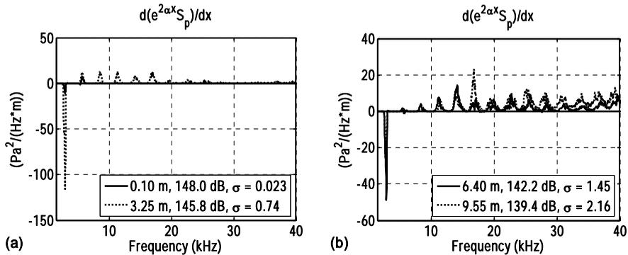
FIGURE 2. Right-hand side of Eq. (2) at four different distances for the same 148 dB source condition.
