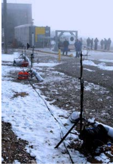
Figure 6a, on the left, shows the three microphone stations and the weather station with the KEI Stage 2 motor in the background. Figure 6b, on the right, shows microphone Station 2. Photo credit ATK.
