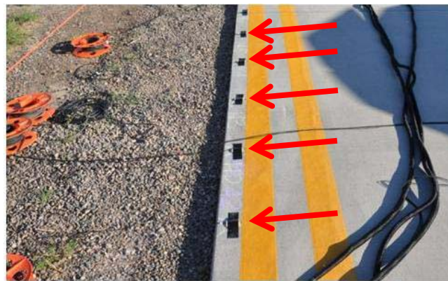
Figure 2 Close-up of several ground-based microphones placed at a perpendicular distance of 11.7 m from the centerline of the jet on an F-22 Raptor. The array spanned more than 30 m.
