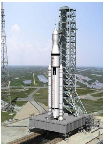
Figure 1. Artist rendering of the proposed SLS vehicle. Note the two five-segment solid rocket boosters.
